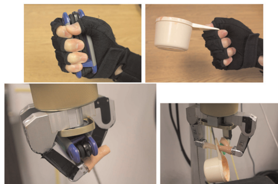
Fig. 1. Corresponding small wrap and lateral pinch of robotic hand to human hand. They look similar to a human grasp but are different for a robotic grasp. Left: Small wrap grasps for a human hand (top) and a robotic hand (bottom). Right: Lateral pinch grasps for a human hand (top) and a robotic hand (bottom).
