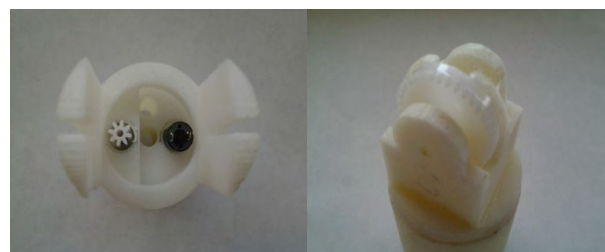
Figure 9. Left: Motor Housing, Right: spurs gear Tilt Cylinder.
