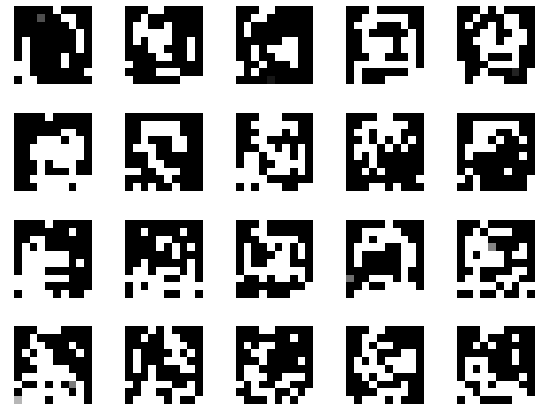
Fig. 9. The top twenty EigenNails for 10 by 10 fingernail images with 6 different directions of force on the fingertip.
