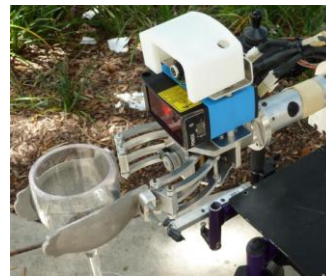
Figure 1. Monocular eye in hand camera mounted on the gripper.
