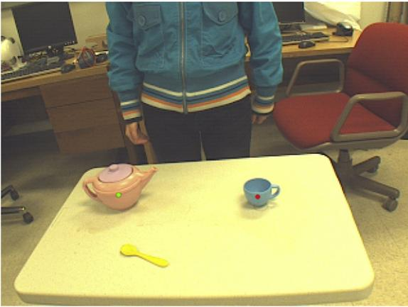
Fig. 4. Example result of object detection with SVM classifier using HoG features. Dots indicate detected object centers.
