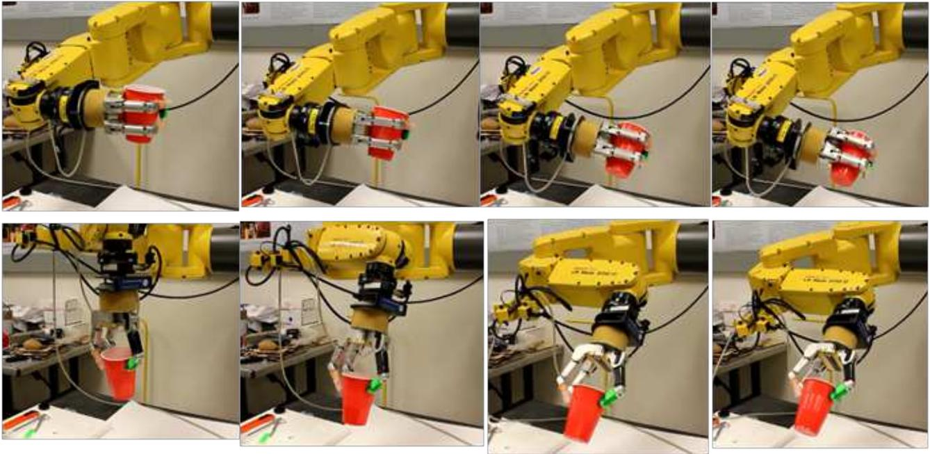
Fig. 7: Compare two different grasps to execute the same manipulation motion of a cup.
