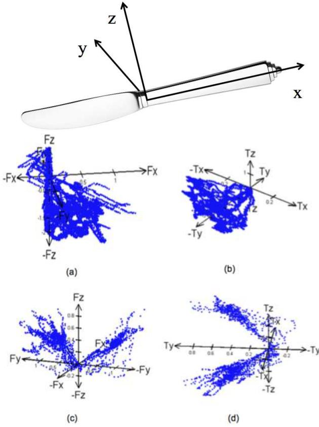
Fig. 3: (a)-(b): cutting task distribution of task wrenches projected to  $F_x$ - $F_y$ - $F_z$  and  $T_x$ - $T_y$ - $T_z$  subspaces, respectively, where the task wrenches are distributed mainly in  $-F_z$  and  $F_x$ ; (c)-(d): corresponding task wrench distribution for butter-spreading task, where the task wrenches are distributed primarily in  $+F_y$ ,  $-F_y$ ,  $+F_z$ ,  $+T_z$ ,  $-T_z$ ;
