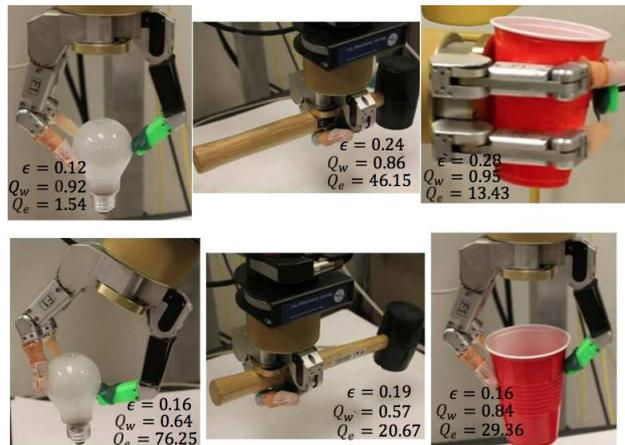
Fig. 6: Example of grasps compared by different quality measures for the three tasks.
