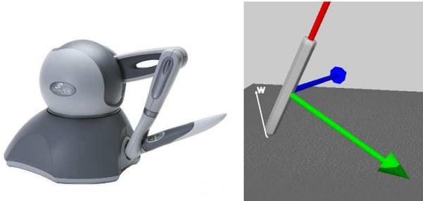
Fig. 1: A user interface for human users to perform manipulation tasks in a virtual environment. Left figure: a haptic device, PHANTOM Omni, to manipulate a virtual instrument. Right figure: a virtual pen is being manipulated in the virtual environment. The motion sequence of the instrument and the disturbance wrench is being captured.
