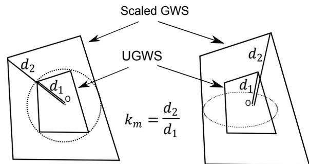
Fig. 2: Grasp quality measures for (a) task ball (b) task ellipsoid.
