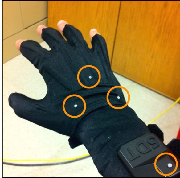
Fig. 3. The 5DT DataGlove 14 Ultra. Notice the encircled passive markers of the MoCap systems used to capture the glove spatial location and orientation.
