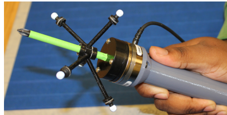
Fig. 1: Instruments are modified for recording interactive motion, force, and torque.
