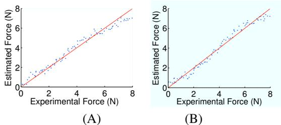
Fig. 6. The estimation result of the GLS model on a new verification data set. (A) The verification result for an index finger; (B) the verification result for a thumb.
