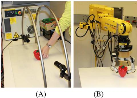
Fig. 4. (A) Grasping force demonstration platform; (B) The robot grasping and manipulation station.
