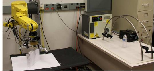
Fig. 2. The robot grasping and manipulation station (left) and the motion and force demonstration station (right) in the grasping force learning from demonstration framework.
