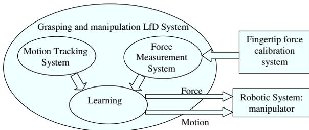
Fig. 1. Presented Framework of grasping and manipulation LfD system.
