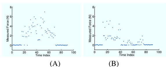
Fig. 8. The measured force by the FlexiForce sensor. (A) the measured force on the index finger; (B) The measured force on the thumb.
