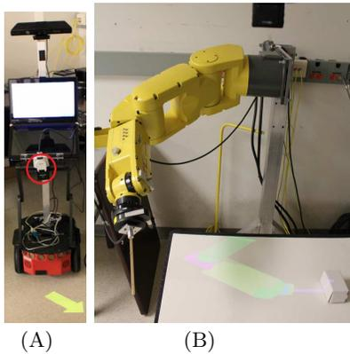
**Figure 1: Telemedicine mobile robot with intention displayed on the floor (A), manipulator with intention displayed with a LASER projector (B).**
